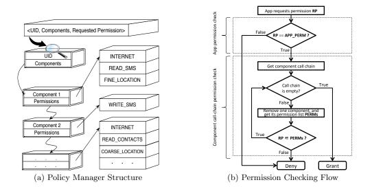
Figure 3: Policy Manager (PM) Structure & Permission Checking Flow
