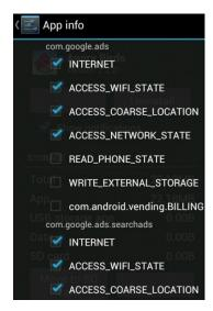
Figure 2: Permission Manager Interface for Users: third-party components with less permissions will be displayed in system settings, and experienced users have options to adjust component permissions in the app info section of system settings.
