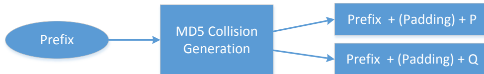
Figure 1: MD5 collision generation from a prefix
